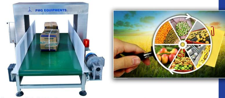
**Conveyor Metal Detectors** are usually manufactured in SS 316 or 304 Finish. It is always customized to the requirement. The tunnel sizes are determined based on the size of the product that has to pass through it. The type of rejection systems is also designed based on the product and operating speeds. PMG is always striving to improve upon its product lines by continuously doing R&D and incorporating it in its products..
